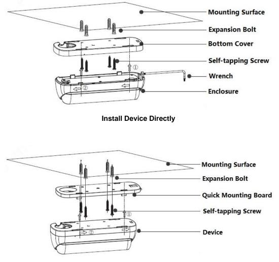
Install Device via Quick Mounting Board
