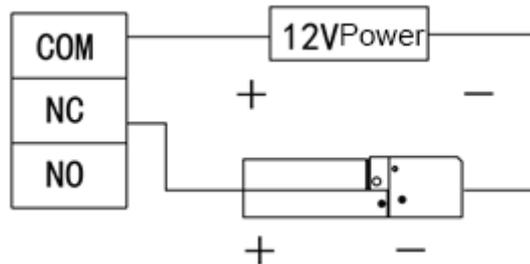
Figure 2-9 Door contact and exit button cable connection
