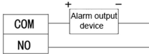
Figure 2-11 Peripheral alarm output device cable connection (2)
