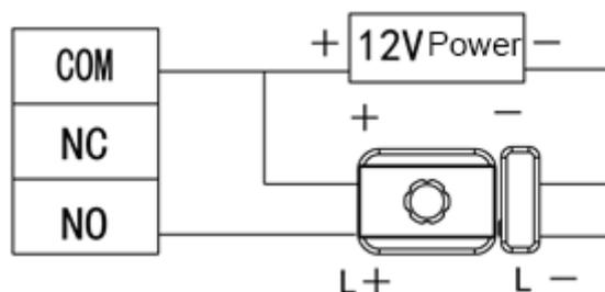
Figure 2-7 Magnetic lock cable connection
