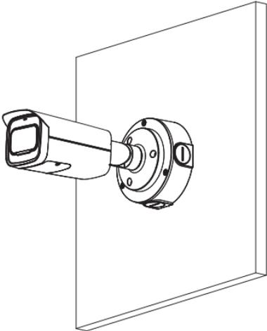
A technical line drawing showing a camera assembly mounted on a flat surface. The camera is a rectangular unit with a lens on the front, connected to a circular mounting bracket. The bracket has a flat base that fits against the surface of the junction box. The junction box is represented as a flat rectangular plate. |
