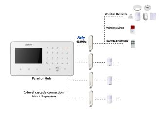
Successfully pair repeater to the panel/hub just like detectors, move repeater to the position between panel/hub and detectors or accessories, then they will search and connect with the repeater automatically
