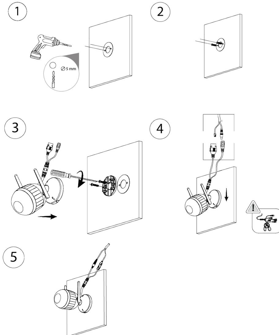
Figure 4-6 Cable going through the mounting surface
