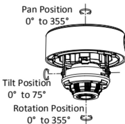
Figure 2-5 3-Axis Adjustment
