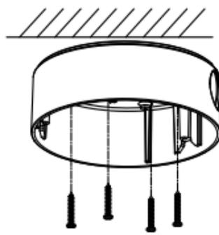
Figure 2-3 Secure the Back Box
