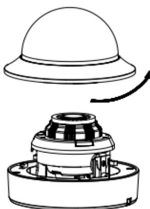
Figure 2-8 Disassemble the Camera
