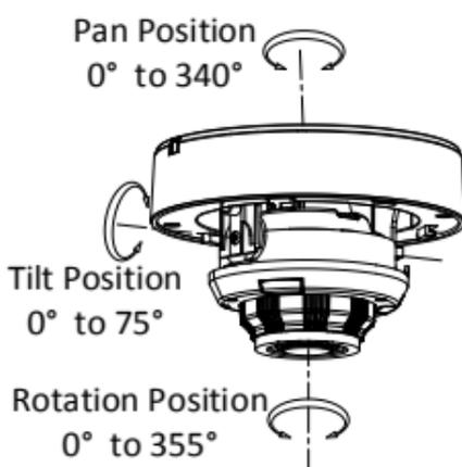
Figure 2-12 3-axis Adjustment
