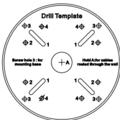
Figure 2-1 The Drill Template
