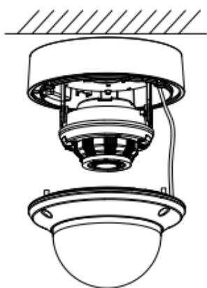
Figure 2-19 Install the Bubble Back
