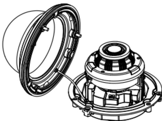
Figure 2-2 Remove the Bubble
