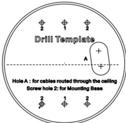
Figure 2-9 The Drill Template
