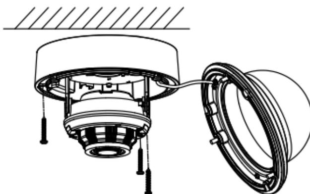
Figure 2-17 Attach the Back Box
