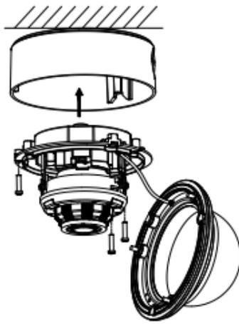
Figure 2-4 Attach the Camera
