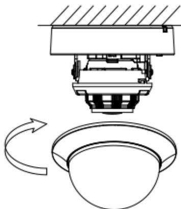
Figure 2-13 Install the Bubble Back
