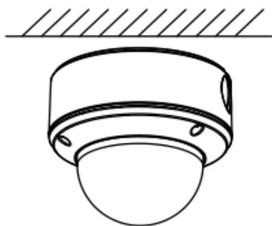
Figure 2-7 Finish Installation
