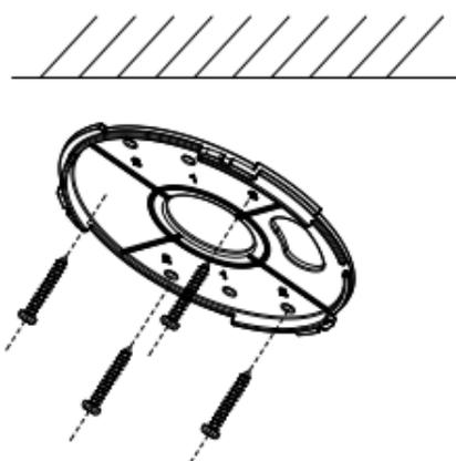
Figure 2-10 Secure the Adapter Plate
