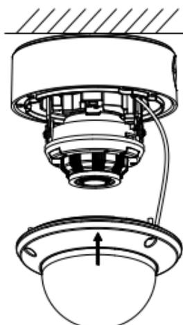
Figure 2-6 Install the Bubble Back
