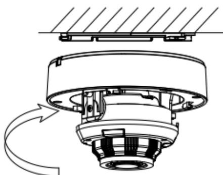
Figure 2-11 Secure the Camera
