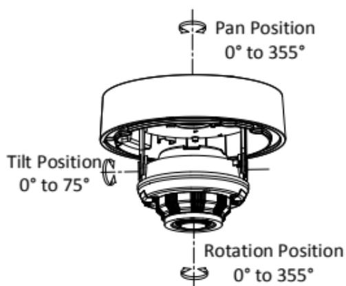
Figure 2-18 3-Axis Adjustment
