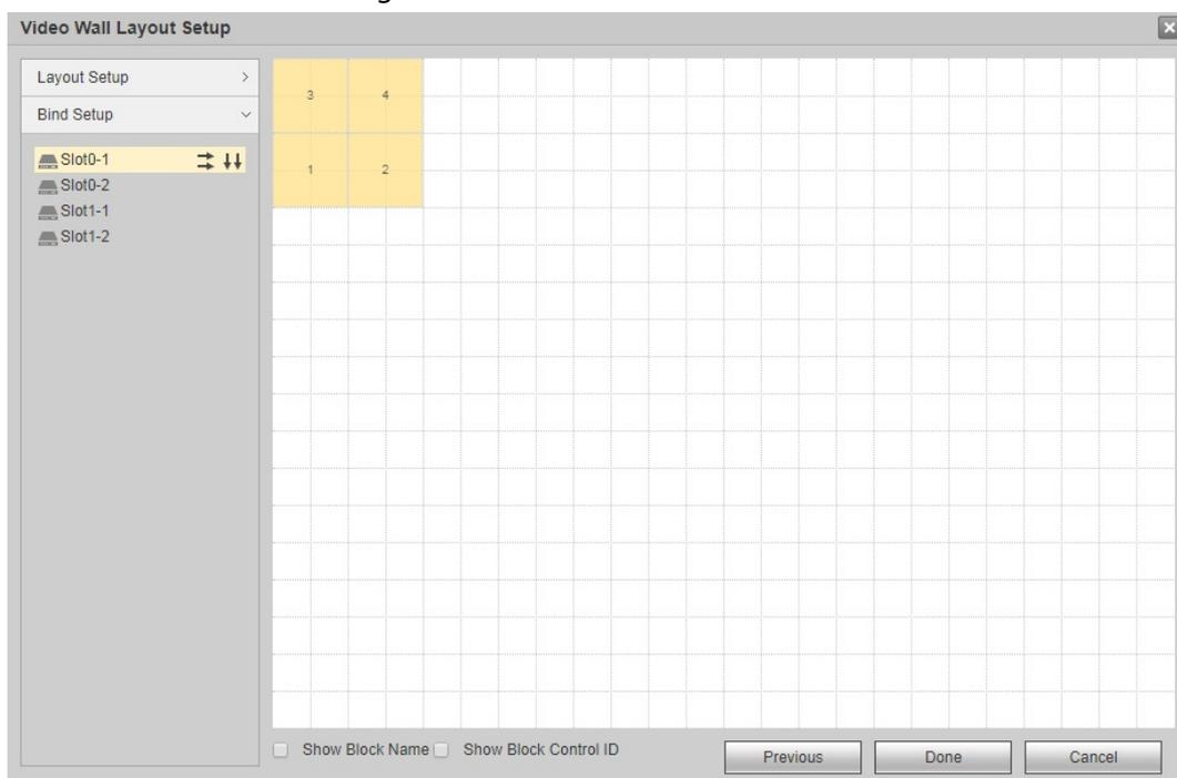
**Step 5** Select one slot, press and hold on left mouse button to drag the slot onto the screen, and bind the slot channel with screen.
