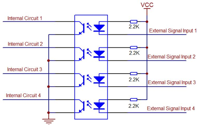
Figure 5-4 Diagram of alarm output port module
