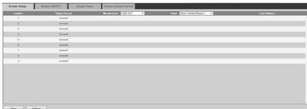
**Step 2** Click drop-down list or text box to configure manufacturer, serial port and com address.
