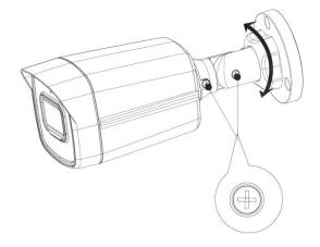
Figure 3-27 Model L adjustment
