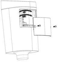
3) Lock the levers and bottom cover, and then fasten the locking screws.
