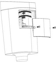
5) Lock the levers and bottom cover, and then fasten the locking screws.
