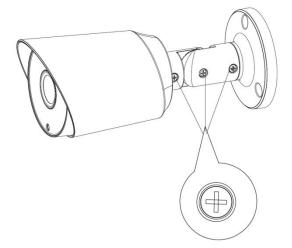
Figure 3-17 Model H adjustment
