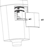
3) Lock the levers and bottom cover, and then fasten the locking screws.
