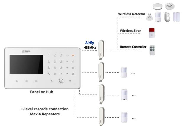
Successfully pair repeater to the panel/hub just like detectors, move repeater to the position between panel/hub and detectors or accessories, then they will search and connect with the repeater automatically
